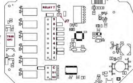
Relay 7 is connected to screw terminals 8 and 9 and can either be a 24 volt or dry contact output. It can be used to indicate occupancy in various ways. Sometimes it is as simple as connecting a light to screw terminals 8 and 9. Sometimes infrared lights and scanners are used so that the hotel staff will know if the room is occupied or unoccupied.
